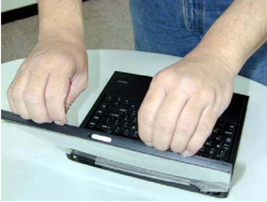
Fig 4-22-01 Removing display mask step (1)
