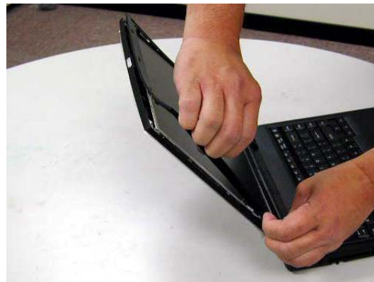
Fig 4-22-04 Removing display mask step (4)
