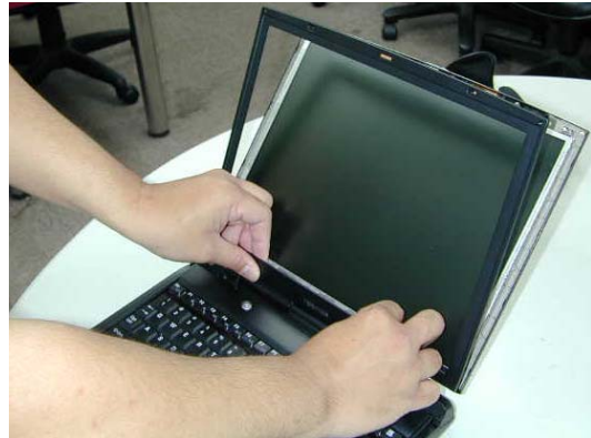
Fig 4-22-06 Removing display mask step (6)
