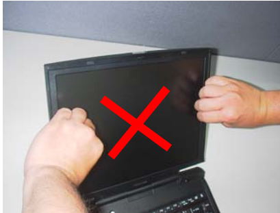
Fig 4-22-08 Removing display mask wrong step (1)
