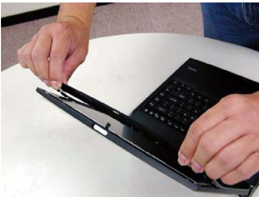
Fig 4-22-03 Removing display mask step (3)
