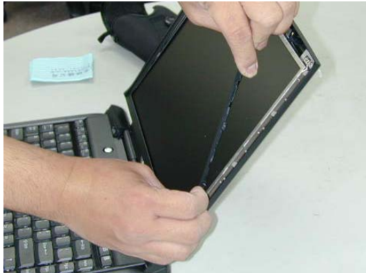
Fig 4-22-05 Removing display mask step (5)
