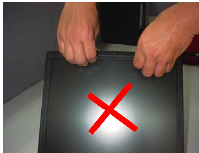
Fig 4-22-10 Removing display mask wrong step (3)
