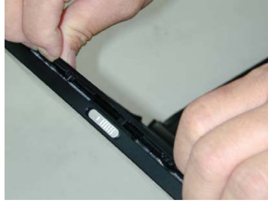
Fig 4-22-02 Removing display mask step (2)
