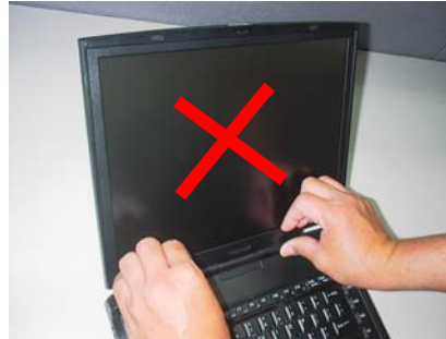
Fig 4-22-09 Removing display mask wrong step (2)
