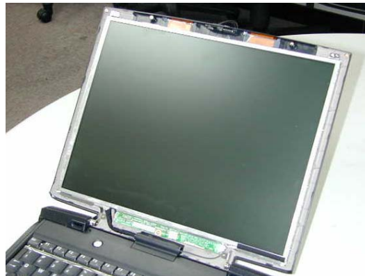
Fig 4-22-07 Removing display mask step (7)
